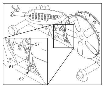
Loosen the M8 x 19mm Flat Head Bolt (61) and turn the Adjustment Screw (62) until the Drive Belt (37) is tight. Once the Drive Belt is tight, tighten the Flat Head Screw.
