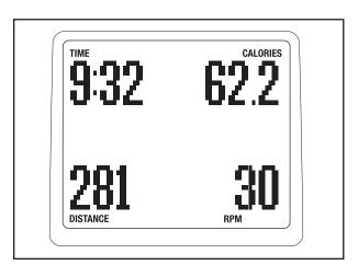
The lower left corner of the display will show the distance (total revolutions) you have pedaled and your power output in watts.
