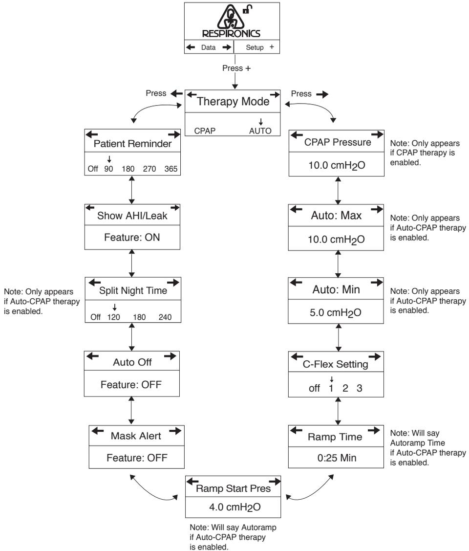
FIGURE 4–7 REMSTAR AUTO M SERIES PROVIDER SETUP SCREENS
