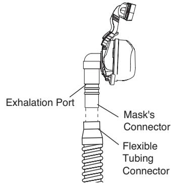
**FIGURE 3–4 CONNECTING A MASK WITH BUILT-IN EXHALATION PORT**
