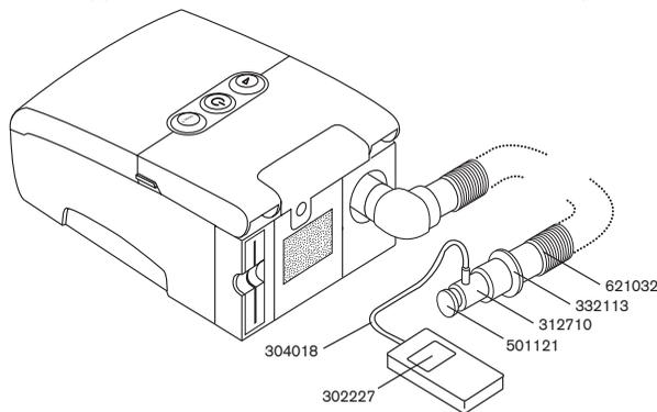
**FIGURE 3–9 CONNECTING THE PRESSURE VERIFICATION EQUIPMENT**
