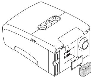
**FIGURE 7-1 REMOVING THE FILTERS**
