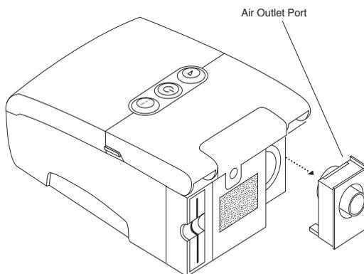
**FIGURE 3-3 DETACHABLE AIR OUTLET PORT**
