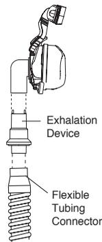
**FIGURE 3–5 CONNECTING A MASK WITH A SEPARATE EXHALATION DEVICE**
