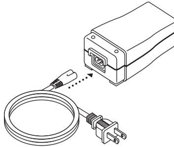
**FIGURE 3–6 CONNECTING THE POWER CORD TO THE POWER SUPPLY**
