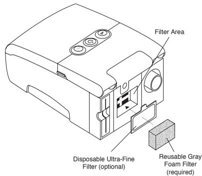
**FIGURE 7-2 REINSTALLING THE FILTERS**
