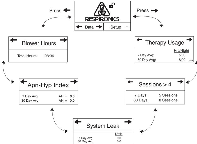
FIGURE 4–6 REMSTAR PRO M SERIES PROVIDER DATA SCREENS
