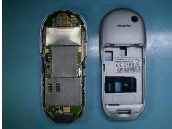
Photo 2.8 Lower case removing
