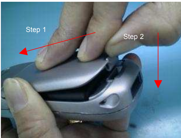
Photo 2.29 Battery cover closing
