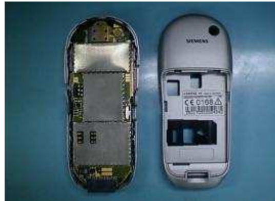
Photo 2.22 RF board placement
