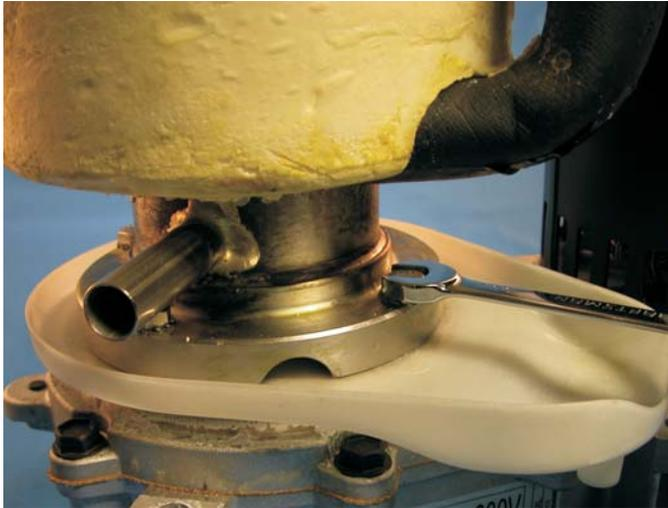
3. Remove the snap ring or wire retainer from the groove under the water seal.
