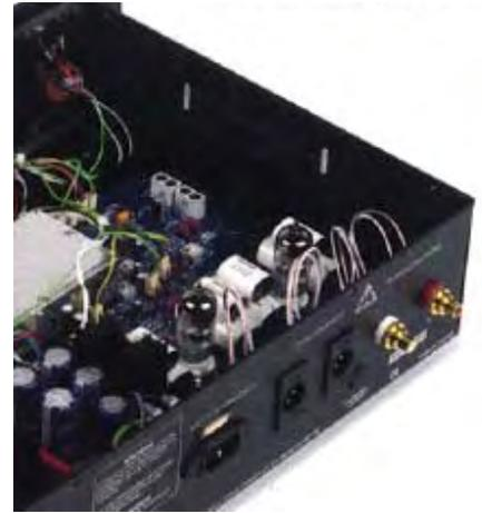
Onix tuners — have sported custom-designed tuner heads. The downside to this custom produced front end is the prohibitive cost. Magnum Dynalab's five-stage tuning front end is entirely custom made and must be one of the last tuners to do so. In the process, this means the method of holding onto a radio signal is now a combination of heavily-shielded toroidal transformer and stabilised power supplies.
