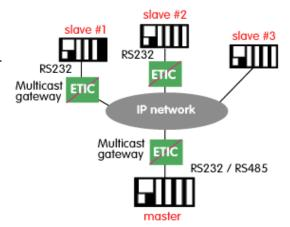
Or when an IP master device (client) has to send requests to multiple slave devices; that devices can be IP or Multicast gateway serial devices.
