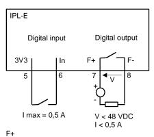
The electrical characteristics of the output are:
