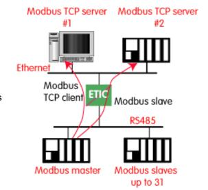
This gateway allows to connect a serial modbus master to the serial interface of the IPRS.
