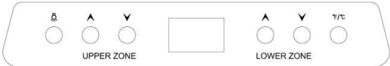
The upper zone temperature can be set between 46° and 54°F. The lower zone can be set between 54° and 64°F. Pressing the “UP” button on the control panel will increase the temperature by 1°F and pressing the “DOWN” button will lower it. Upon choosing your desired temperature, the display will flash the selected temperature setting for 5 seconds before reflecting the current internal cabinet temperature.
