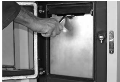
Fig. 5 Pulling up the heat shield and hooking it into the lugs on the sides
