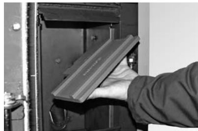
Fig. 82 Removing and cleaning the baffle plate
