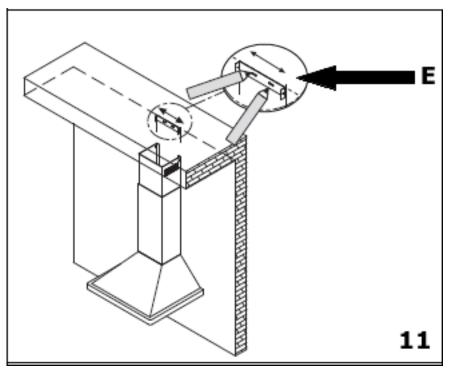
**11)** Take the fixing bracket ( $\mathbf{E}$ ) and place it between the two pencil marks that you made in step 9
