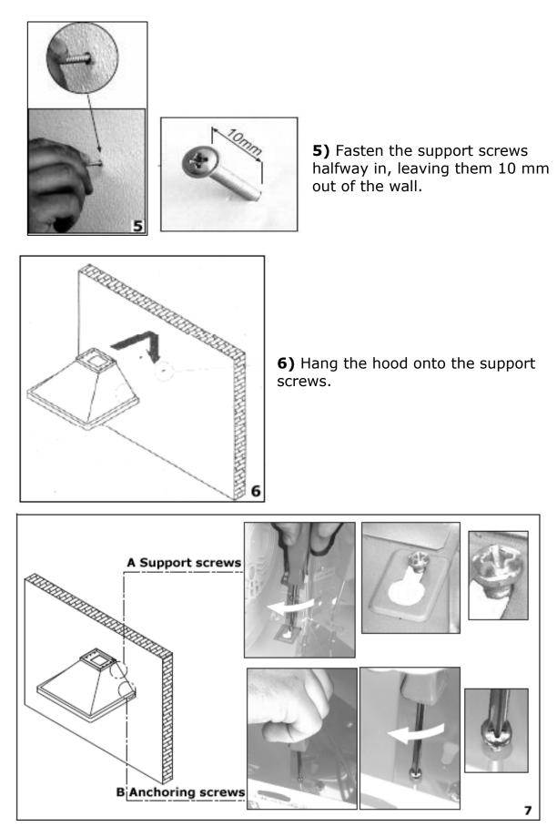
**7)** Fully tighten the support screws **(A)** and then screw the anchoring screws **(B)** through the relevant holes in the cooker hood. Fully tighten the anchoring screws fully into the wall.
