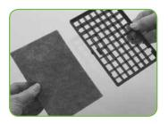
Remove the motor filter from its carrier and wash under warm tap water. Dry thoroughly and refit.
