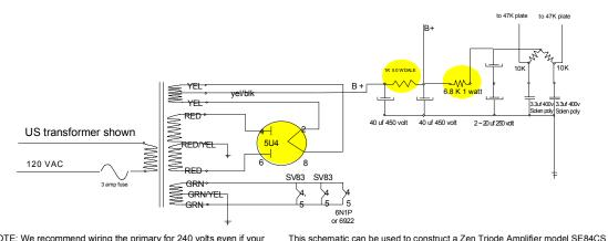
NOTE: We recommend wiring the primary for 240 volts even if your voltage is 220 or 230. Use a 3 amp fuse.
