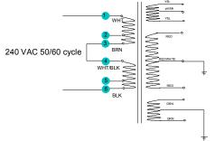
For Japan 100 volt connect 1 to 4 and 2 to 5 Use 1,4 and 2,5 for line connection.
