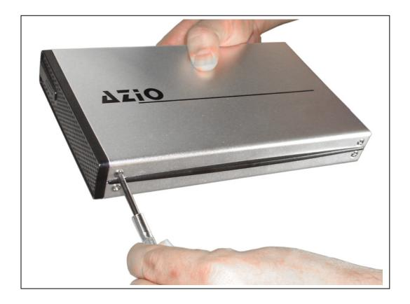
Open the drive kit by carefully remove the top cover from the body chassis.
