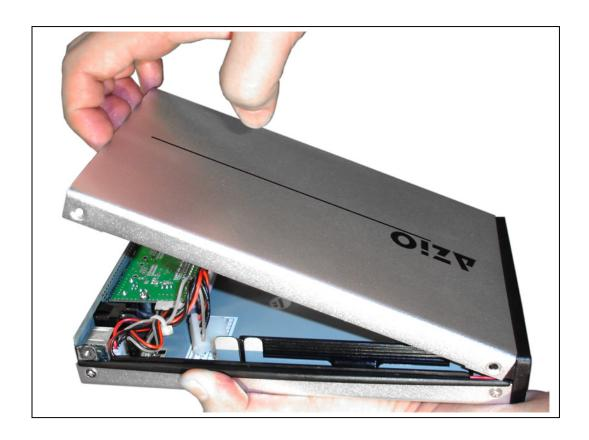
**Warning:** When handling the opened kit, never touch the PCB (printed circuit board). It contains sensitive electronics that can be easily damaged.
