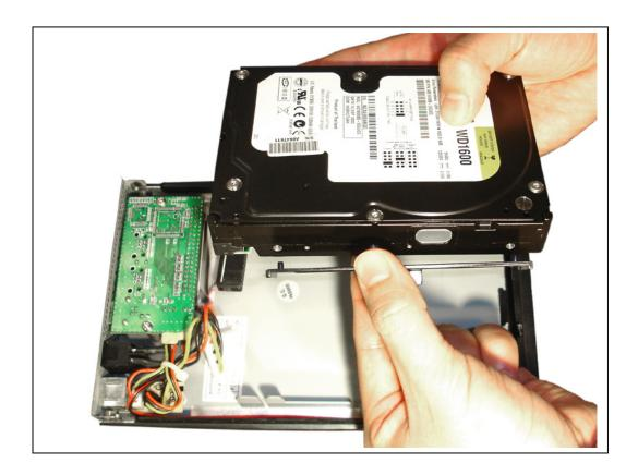
While holding on to the hard drive brackets, connect the power and flatribbon IDE cables to the drive. For SATA drives, there will not be a flatribbon cable. Simply install the hard drive into the interface connector. Insert the drive unit onto the bottom chassis of the drive kit.
