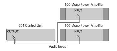
Connect the sockets marked OUTPUT L and R on the back panel of the 501 Control Unit to the INPUT socket on the back panel of each of the 505 Mono Power Amplifiers.
