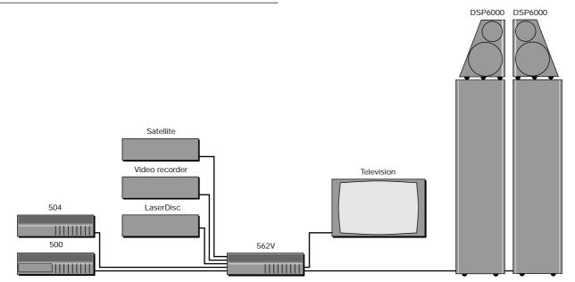
The 562V Multimedia Controller is the ideal control unit for use with the Meridian DSP6000 Digital Loudspeakers.
