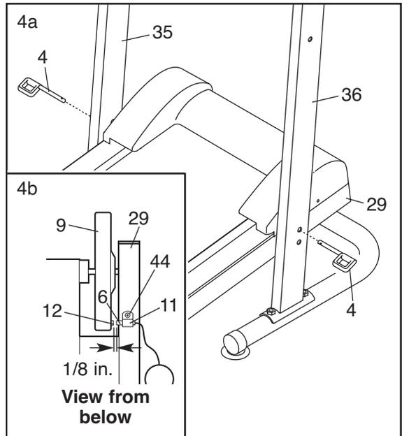
Look under the Frame (29) near the Left Upright (35). **See drawing 4b.** Locate the Reed Switch Clip (11) attached to the underside of the Frame. Insert the Reed Switch (6) into the Clip as shown. Next, locate the Magnet (12) on the left Flywheel (9). Turn the Flywheel until the Magnet is aligned with the Reed Switch. **Move the Reed Switch so that there is a 1/8" (3 mm) gap between the Reed Switch and the Magnet.** Then, tighten the M5 x 12mm Screw (44) in the Clip.
