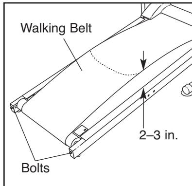
hex key, turn both rear roller adjustment bolts counterclockwise 1/4 of a turn. When the walking belt is properly tightened, you should be able to lift each edge of the walking belt 2 to 3 in. (5 to 7 cm) off the walking platform. Be careful to keep the walking belt centered. Walk on the treadmill for a few minutes. Repeat until the walking belt is properly tightened.
