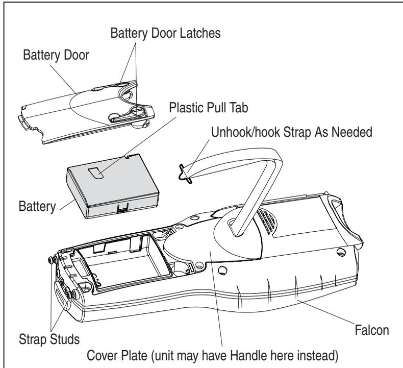
2. Turn the battery door latches to unlock the battery door. Remove the door.
