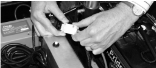
Figure 20. Disconnecting The Front-to- Rear Harness
