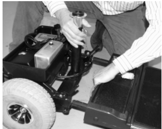
Figure 26. Separating The Frame
