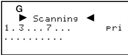
2. Numbers represent active scan lists, periods represent inactive scan lists. To toggle a list, press the corresponding number on the keypad. For 11-20, press **FUNC** and then the second number (**FUNC + 3 = 13**).
