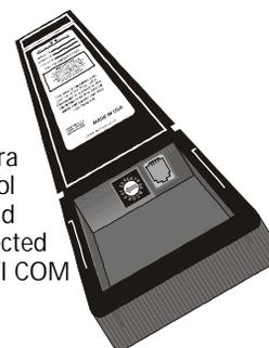
Camera Control Keypad connected via PVI COM Port
