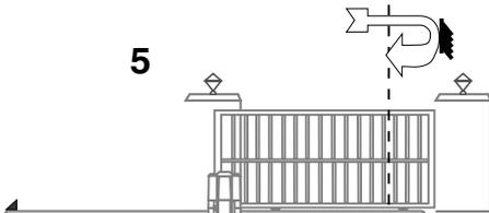
5 - As gate sensor passes the motor, the speed reduces to CRAWL. Gate hits "closed" end stops and reverses at FULL SPEED.
