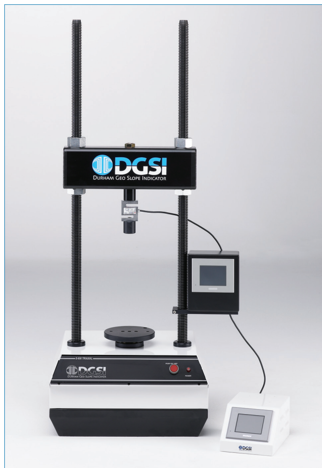
S-600 shown with S-type Load Cell and EZ-Daq data acquisition system (sold separately).
