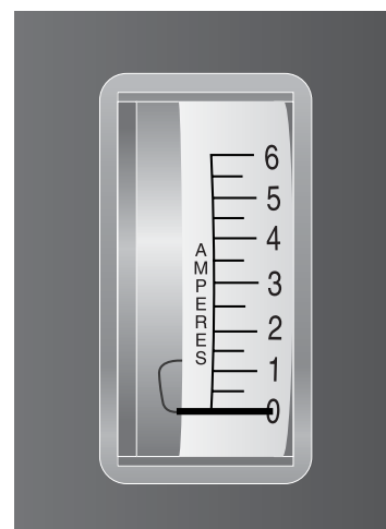
FIGURE 12. AMMETER INDICATES BATTERY IS FULLY CHARGED
