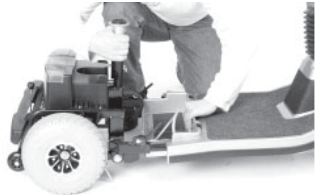
FIGURE 25. SEPARATING THE FRAME SECTIONS
