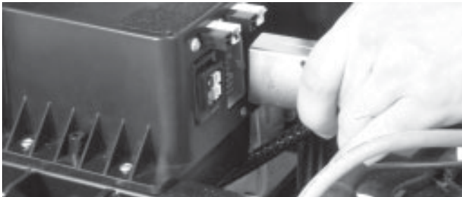
FIGURE 21. DISCONNECTING THE FRONT-TO-REAR HARNESS
