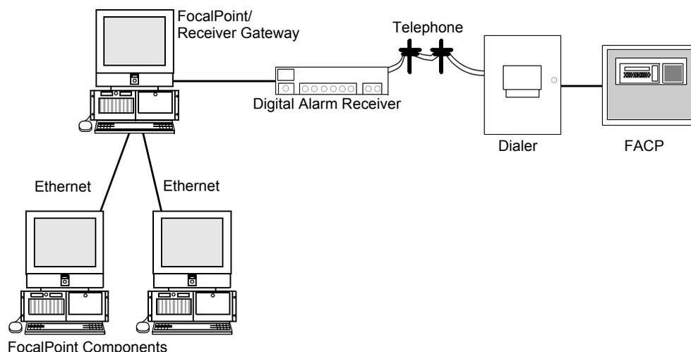
Figure 1.2 Receivers Telephone Architecture Diagram
