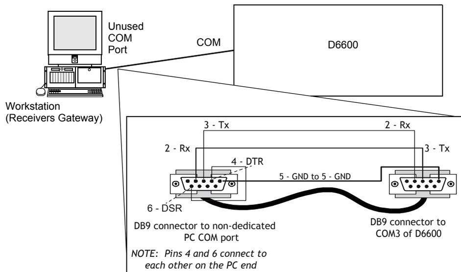
Figure 2.3 D6600 To Gateway Serial Connection
