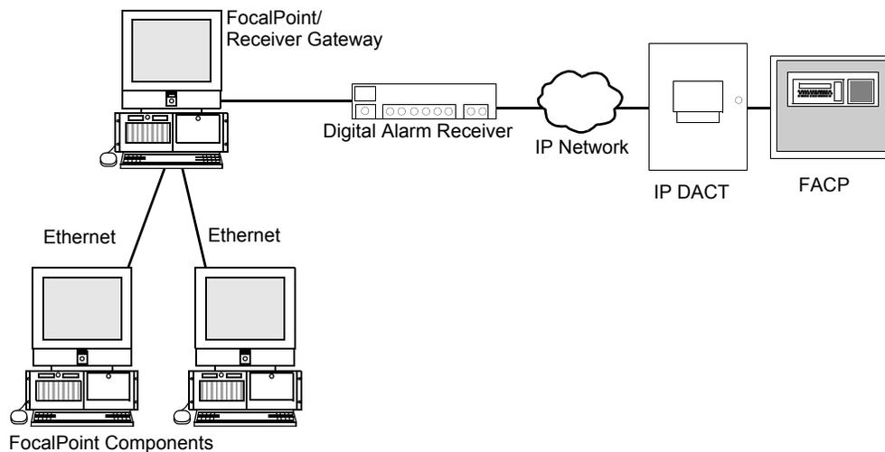
**Figure 1.1 Receivers IP Network Architecture Diagram**
