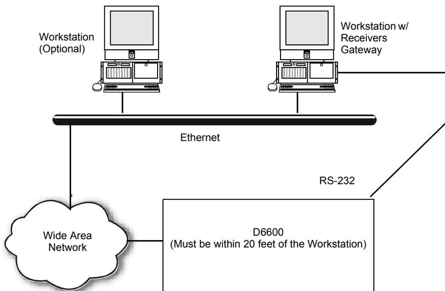
Figure 2.2 Radionics D6600 Receiver Application Example
