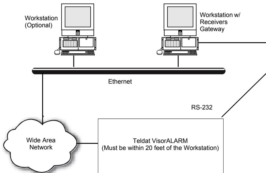
Figure 2.6 Teldat VisorALARM Receiver Application Example
