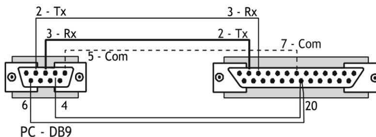
Figure 2.5 VisorALARM Cable Connections
