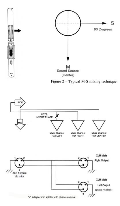
Figure 3 – Typical M-S connection set-up
