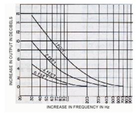
Typical relationship of microphone distance to frequency response for ribbon-velocity bidirectional microphone.
