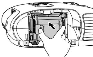
**7** Securely tighten the lamp fixing screws.
