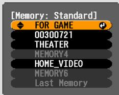
Press or on the remote control or or on the projector's control panel to select an item.
