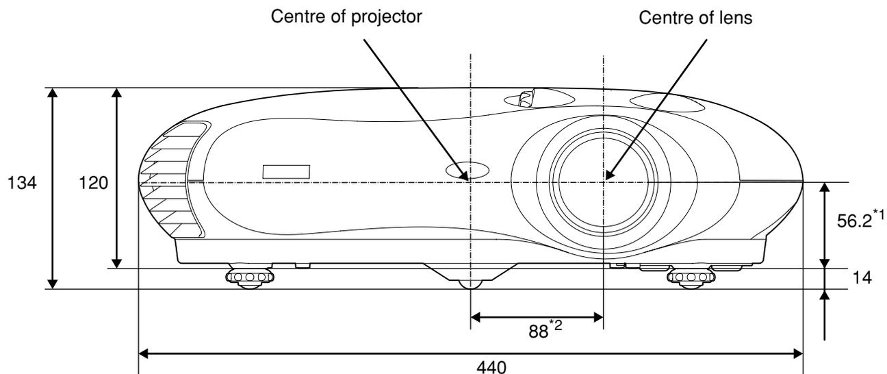
\*1 Distance from centre of lens to suspension bracket fixing point
