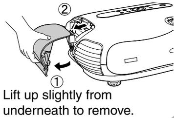
Lift up slightly from underneath to remove.
