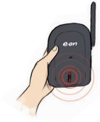
When you release the button, you'll see a red light on the transmitter flashing rapidly - this means it's ready to 'tune' itself with your monitor.
