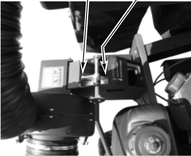
Figure 8 Belt Tension Rod Cam Stop Bolt Is Below The Cam Assembly
