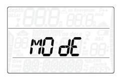
Here you can define the type of gas you will be breathing during the dive (air or enriched air nitrox, including multigas). You can also set Nemo Wide to bottom timer, in which case Nemo Wide will show only time, depth and temperature: it will not carry out any decompression calculation and it will not show any warnings and alarms.
