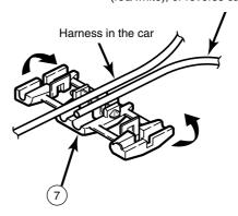
Press down the cover of the splicing connector and squeeze it until it locks.
