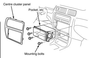
■ If installing using the 2DIN installation kit (sold separately)
