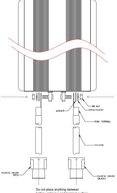
Do not place anything between battery cable lug and terminal surface. Assemble exactly as shown.
