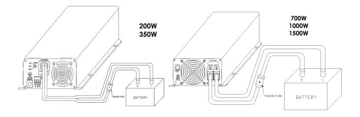
Battery to inverter cable connection
