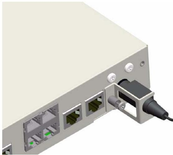
**Figure 1: Connecting the Power Brick on OmniAccess 5510 USG**
