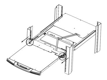
4. Using the front handle, push the module all the way in until it clicks into place.
