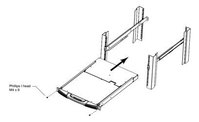
4. Slide the rear attachment sliding brackets along the slide bars until they contact the rear of the switch, then use the screws supplied with this package to attach the bars to the rear of the switch (tighten the screws all the way).
