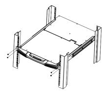
2. While the first person still holds the switch in place, the second person slides the L brackets into the switch's side mounting brackets, from the rear until the bracket flanges contact the rack, then - using the screws provided with the rack mounting kit - screws the L brackets to the rack.
