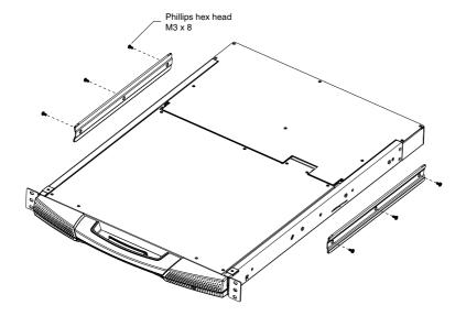
2. Attach the left and right *easy-installation* mounting rails to the inside of the rack. The flange that supports the switch will be to the inside.
