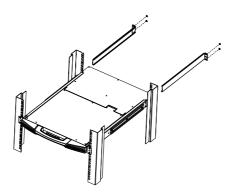
3. After the L brackets have been secured, tighten the front bracket screws
