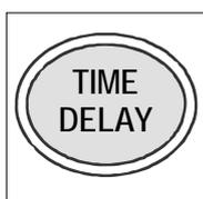
Press this pad to select the time you wish the washing to be completed. Example: If it is 8.00 am and you wish the wash to be completed at 5.00pm press the button 9 times . i.e. one press for each hour delay. The display will indicate your selection. The wash will be completed by the end of the selected time.
