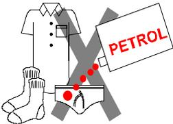
Do not wash clothes soaked in petrol, thinners, vegetable oil or any other flammable liquids. Nor should any of these liquids be added to the wash water as they constitute a fire hazard.
