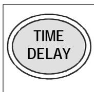
Press the TIME DELAY pad as many times as you require. The digital display shows the delay time. Every press of the pad delays the completion time by one hour.
