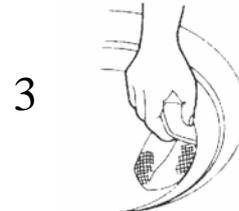
Re-shape the filter mesh and fit the filter frame back in it's slot.
