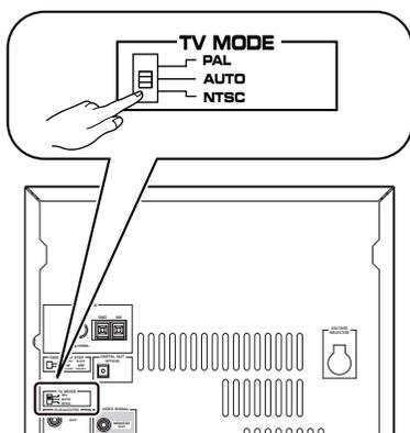
This system is designed for use with the NTSC and PAL television formats. Set this switch to the position of the format your TV monitor employs.
