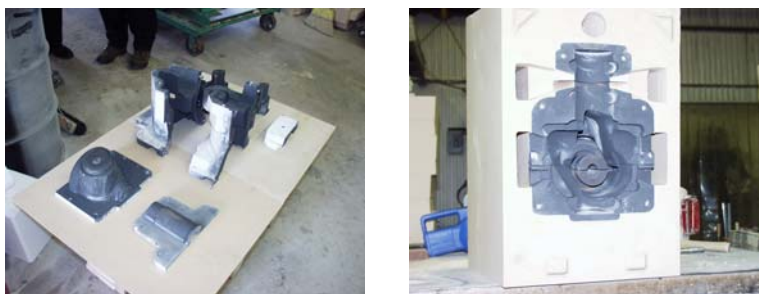
Figure 4: Shell Method – ZCast components of a shell mold (left). Assembled mold with ZCast components packed in foundry sand. Note that the risers, runners and sprue have been formed in the foundry sand (right).
