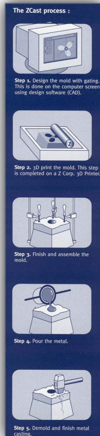
Figure 5: Steps involved in using ZCast powder
