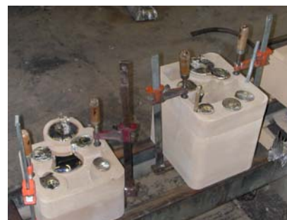
Figure 3: Direct pour molds in aluminum after pouring (note significant number of risers).
