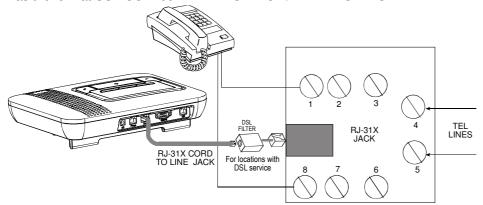
Note: For whole house line seizure with DSL service present on the phone line, you must install a filter. It is suggested to use the DSL alarm filter model Z-A431PJ31X manufactured by Excelsus Technologies, or equivalent. This filter simply plugs into the RJ-31X jack and allows alarm reporting without breaking the internet connection.
