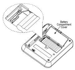
Figure 6 – Replacing the Battery
