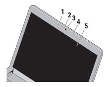
1 Left digital array microphone – Combines with the right digital array microphone to provide high quality sound for video chatting and voice recording.
