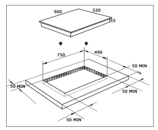
Cut a hole in the worktop that corresponds with the drawing shown above.
