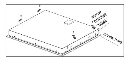
Carefully turn the hob back over and then gently lower it into the aperture hole that you have cut out.
