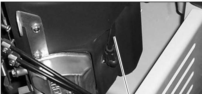
2. Clean the electrodes by scraping with a wire brush to remove carbon deposits.
