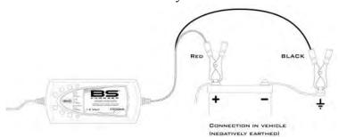
o If Positively Earthed – FIRST Connect the Black (-) battery charger lead to the Negative (-) battery post and then connect the Red (+) battery charger lead to the Vehicle's chassis and far away from the fuel line.
