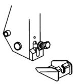
When mounting for the first time, the front hook bolts will have to be tightened after positioning the hook directly over the mounting boss (most rearward position)
