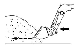
Note: Bottom surface of bucket is parallel to line on motion.
