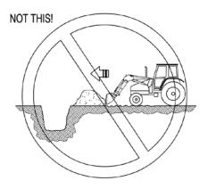
Do not use bucket in dumped position for bulldozing. This will only impose severe shock loading on the bucket cylinders and make it more difficult to maintain a level grade.
