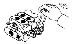
Work both levers back to direct pressure to both cylinders.
