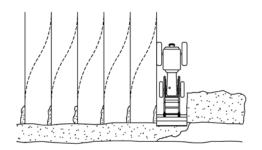
Leave material, which drifts over the bucket sides for final cleanup.
