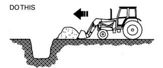
When backfilling approach pile with a flat bucket. Leave dirt in bucket. Dumping on each pass wastes time.
