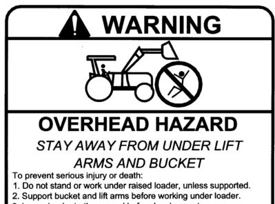
3. Lower loader to the ground before leaving seat.
