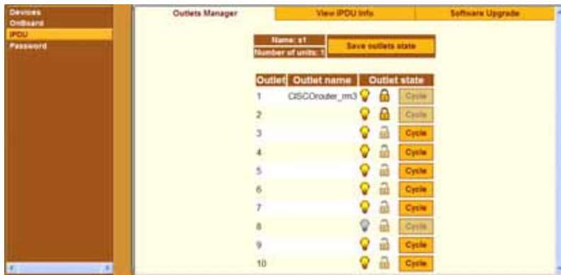
Figure 3.16: Access - IPDU - Outlets Manager Screen
