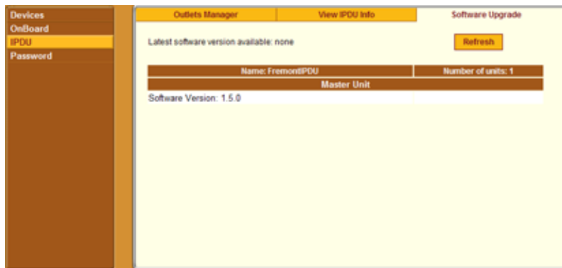
Figure 3.19: IPDU Software Upgrade Screen on the Web Manager
