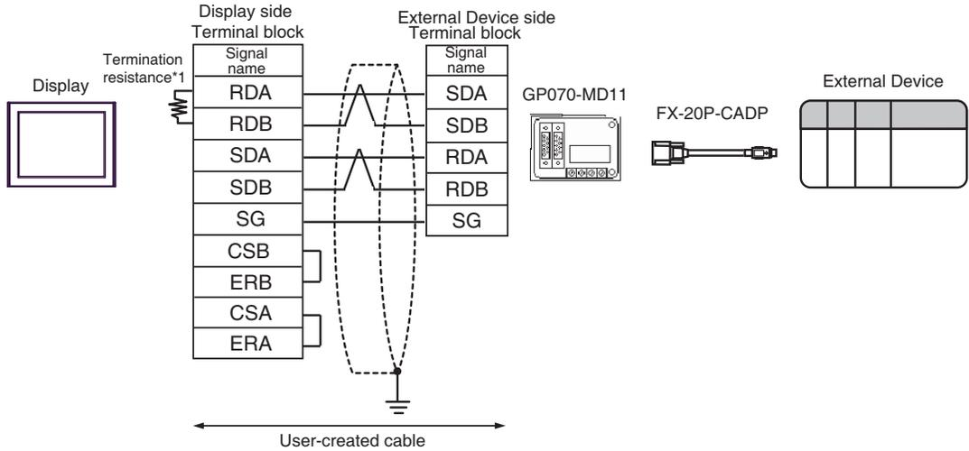
\*1 The resistance in the Display is used as the termination resistance. Set the value of the DIP Switch on the rear of the Display as shown in the table below.
