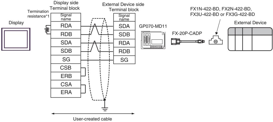
\*1 The resistance in the Display is used as the termination resistance. Set the value of the DIP Switch on the rear of the Display as shown in the table below.
