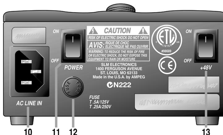
**10. AC LINE IN:** The grounded power cord should only be plugged into a grounded power outlet that meets all applicable electrical codes and is compatible with the voltage, power and frequency requirements stated on the rear panel. **Do not attempt to defeat the safety ground connection!**
