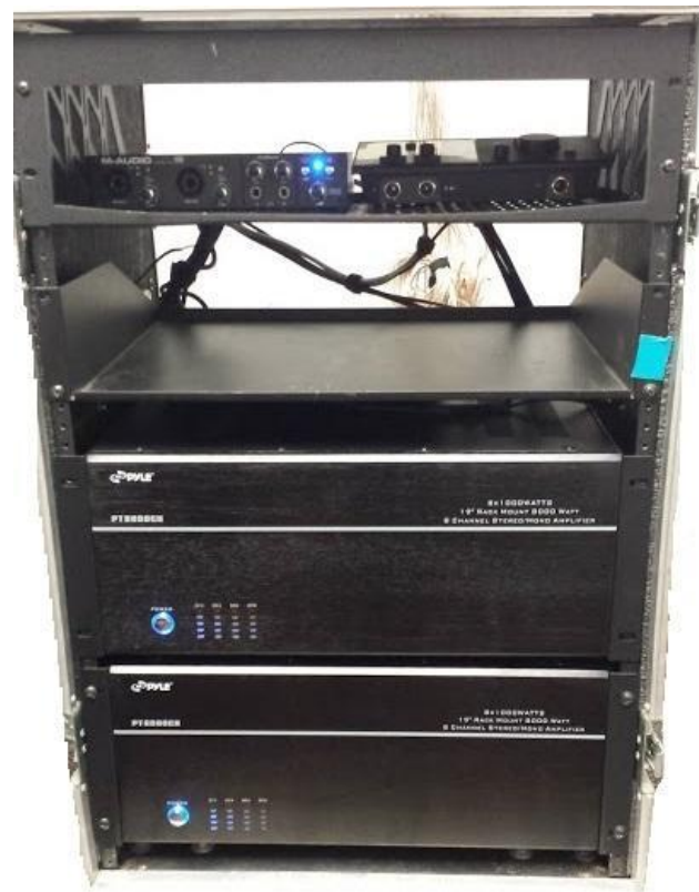
Figure 19: Profire 610 (top left) and Fast Track C400 Interfaces(top right) and Pyle Amplifiers in Audio Rack (bottom)
