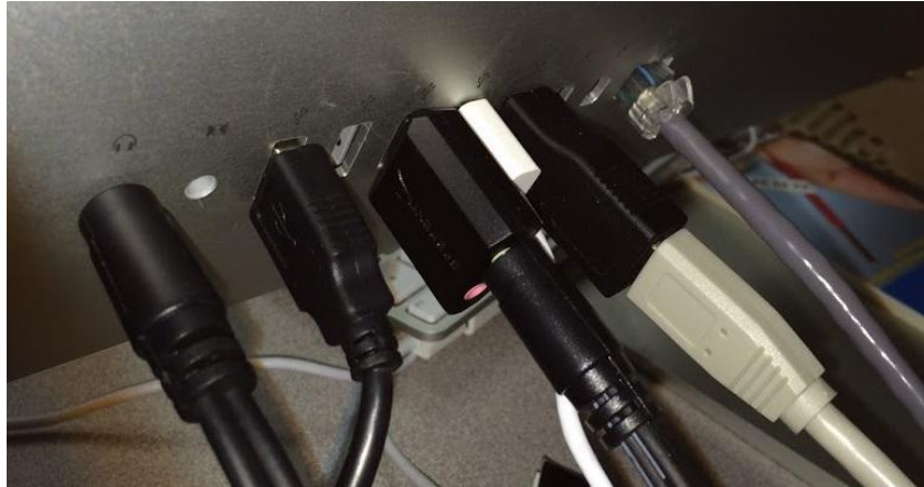
Figure 20: Connections to iMac including (from the left) 3.5mm headphone jack, USB to Profire 610, Syba USB, and USB/Firewire to Fast Track
