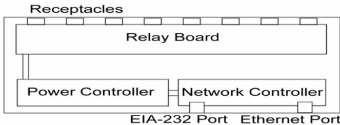
**Power Controller:** The power controller connects to the relay board to control the outlets. EIA-232 Port maybe on either controller.
