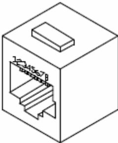
**Fig. 1: RJ-45 Receptacle**
