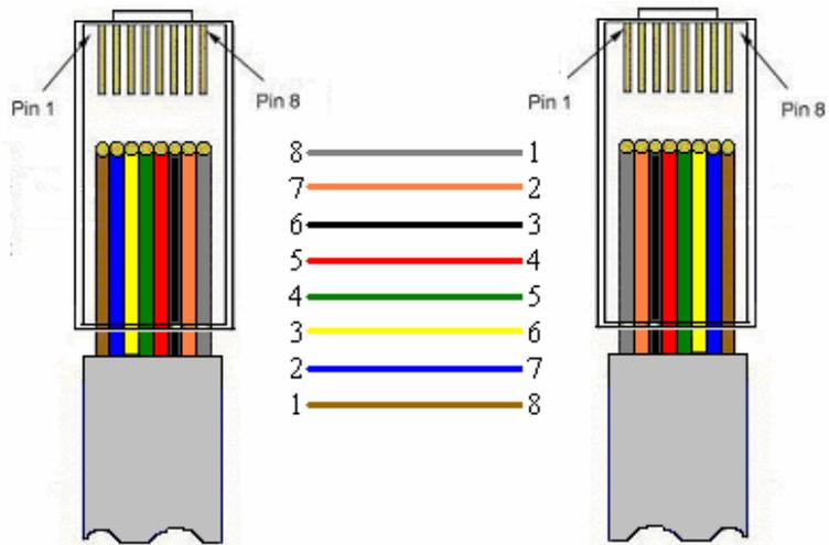
Figures 1 and 2 provide visual representation of an RJ-45 receptacle and plug.
