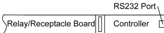
**Power Controller:** The power controller connects to the relay board to control the outlets. EIA-232 located on Controller.
