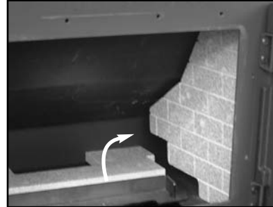
Fig. 3c Fitting the side linings
