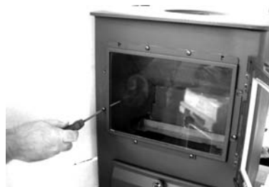
Fig. 12 Removing the Glass Frame
