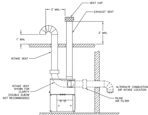
Fig. 27: Direct Vent - Vertical
