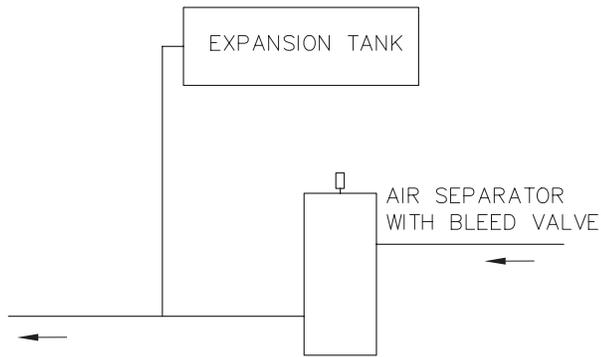
Fig. 9: Air-Separation/Expansion Tank
