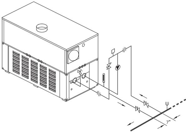
Fig. 13: Single Pool Heater Application
