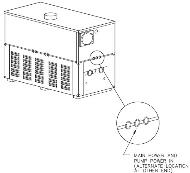
**Fig. 19: Wiring Location**
