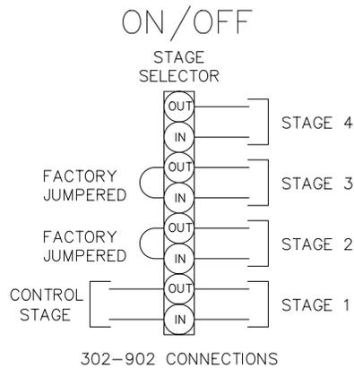
**Fig. 20: On-Off Wiring Connections**
