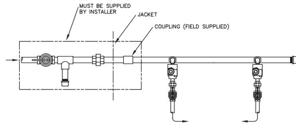
**Fig. 15: Gas Supply Connection**
