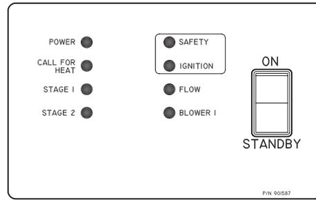
Fig. 28: External LED Indicator Decal
