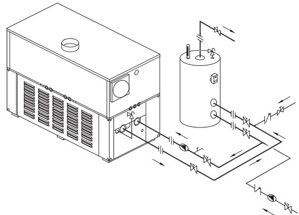
**Fig. 12: Single Domestic Hot Water Heater and Storage Tank**
