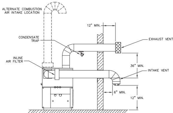
Fig. 39: Direct Vent - Horizontal Through-the-Wall
