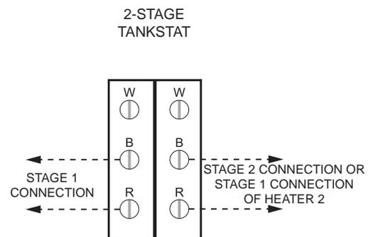
ATTACH STAGE 1 CONNECTIONS ON HEATER TO STAGE 1 CONNECTION ON TANKSTAT.
