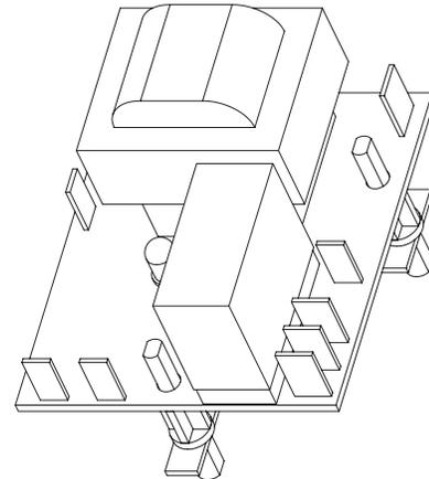
Fig. 33: Low Water Cut-Off
