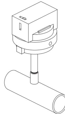
Fig. 34: High/Low Gas Pressure Switch
