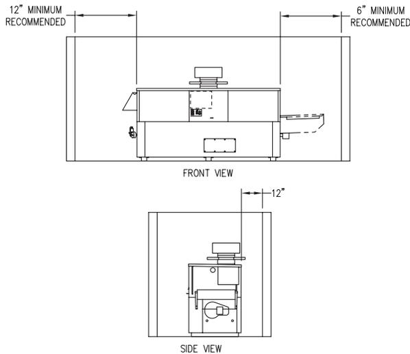
**Fig. 7: Minimum Clearances from Combustible Surfaces – Outdoor Installations**
