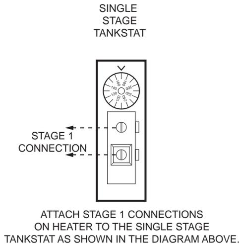
**Fig. 23: Single-Stage Tankstat**
