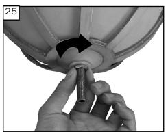
Place glass and cage on light kit, install rubber washer and hex nut to hold in place and tighten in direction of arrow.
