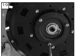
Loosen 2 screws and remove 1 screw. Save screw removed.
