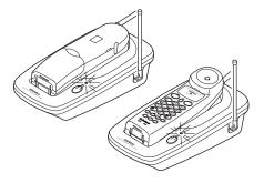
Recharge the battery pack when the handset beeps and the TALK/BATT indicator flashes.
