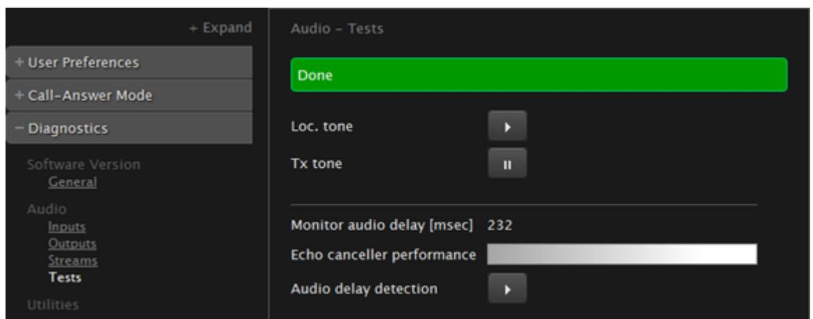
4. Select the Tx tone button to check the audio output. If the test is completed successfully, the Done message is displayed.
