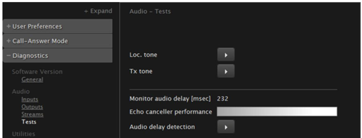
3. Select the Loc tone button to run the audio input. If the test is completed successfully, the Done message is displayed.
