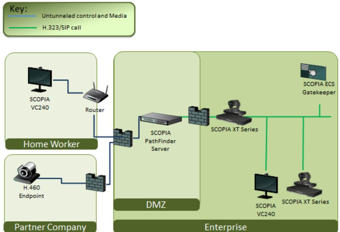
Configure the traversal server as the XT Codec Unit gatekeeper and enable the H.460 option. Configure the XT Codec Unit to the IP address of the traversal server SCOPIA PathFinder.
